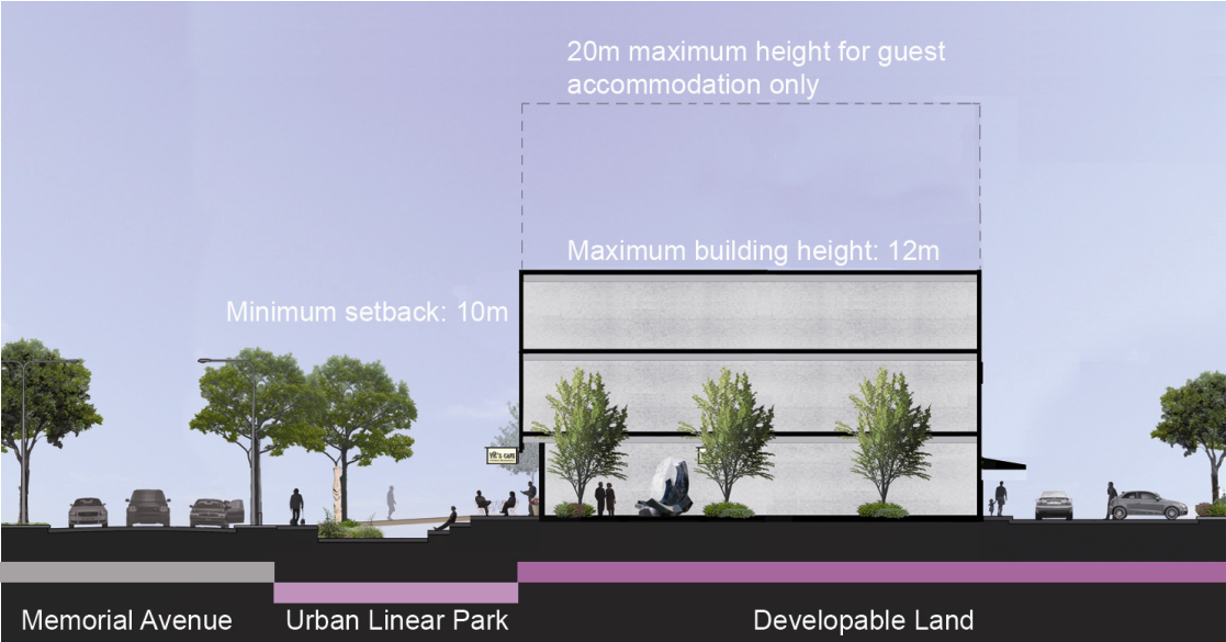
Section 1: Memorial Avenue Proposed Edge Condition
