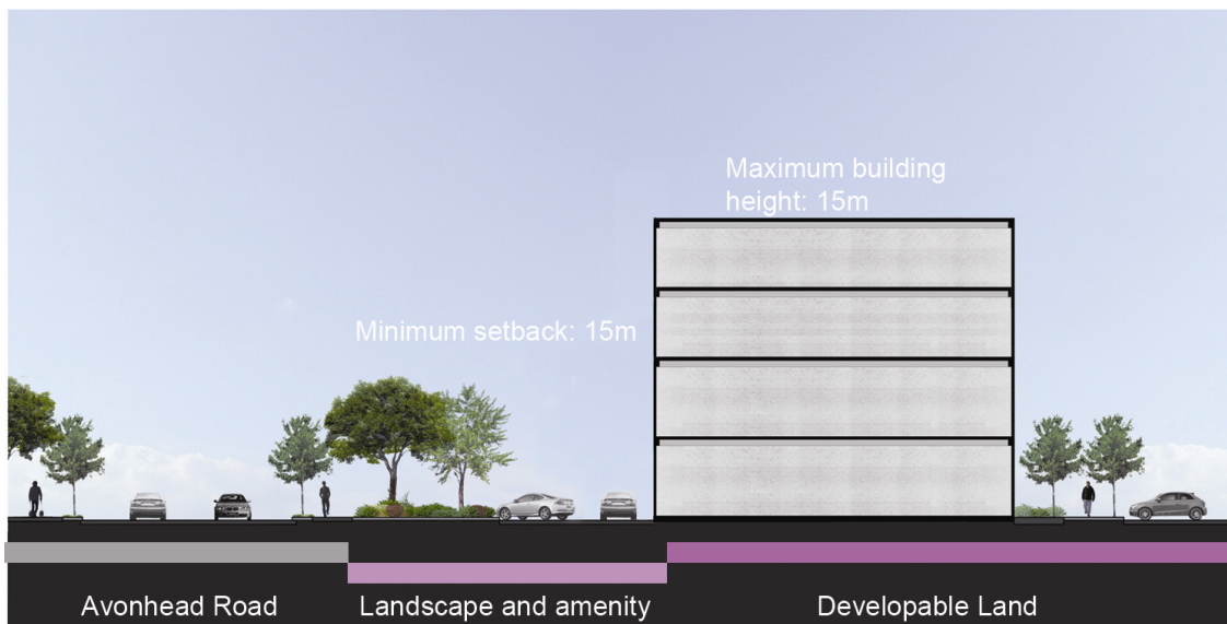
Section 3: Avonhead Road Proposed Edge Condition
