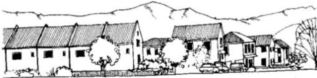
Figure 2: Townhouse block demonstrating overly repetitive elements. The buildings to the right display a pleasing variety and interest.
