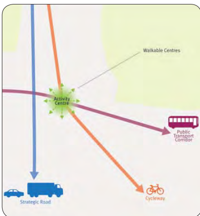
Figure 5.2. Concept of an integrated transport network. Each mode will travel on a designated road - different roads for different purposes.
