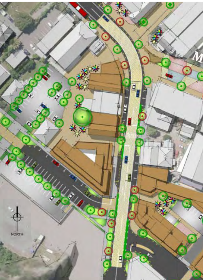
Figure 43. Option 2 – plan view for the design of Marriner Street / Wakefield Avenue with increased extent of paved area
