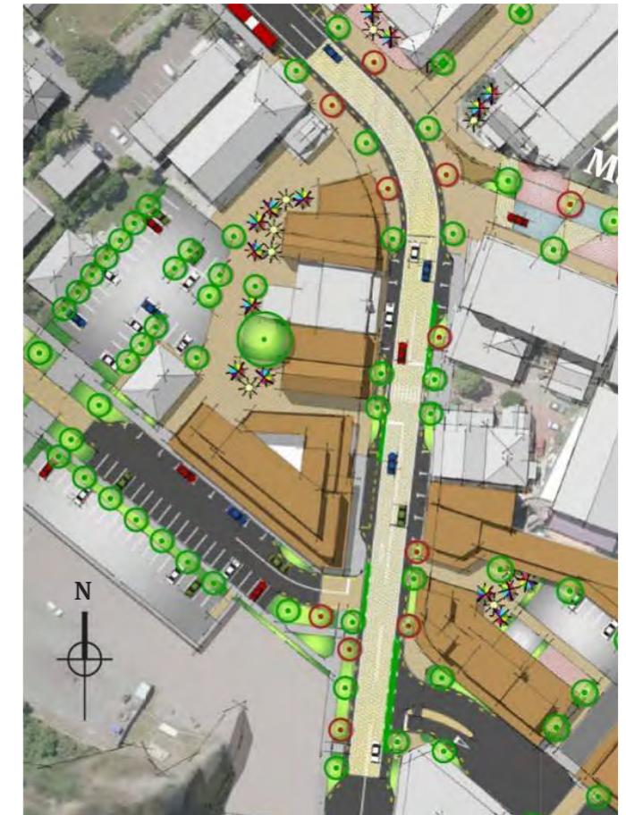
Figure 9. Option 2-plan view for the design of Marriner Street/Wakefield Avenue with increased extent of paved area
