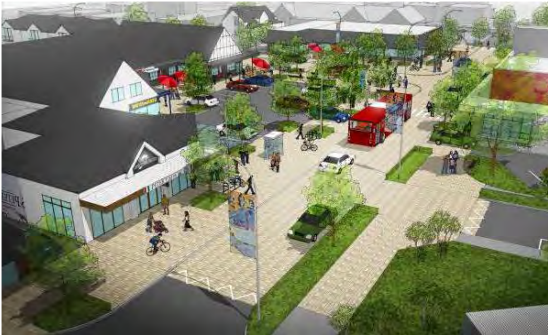
Figure 6b – view along Edgeware Road, showing road platform and pedestrian priority
