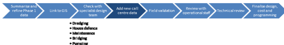
Figure 4 Local area and maintenance scheme design process
