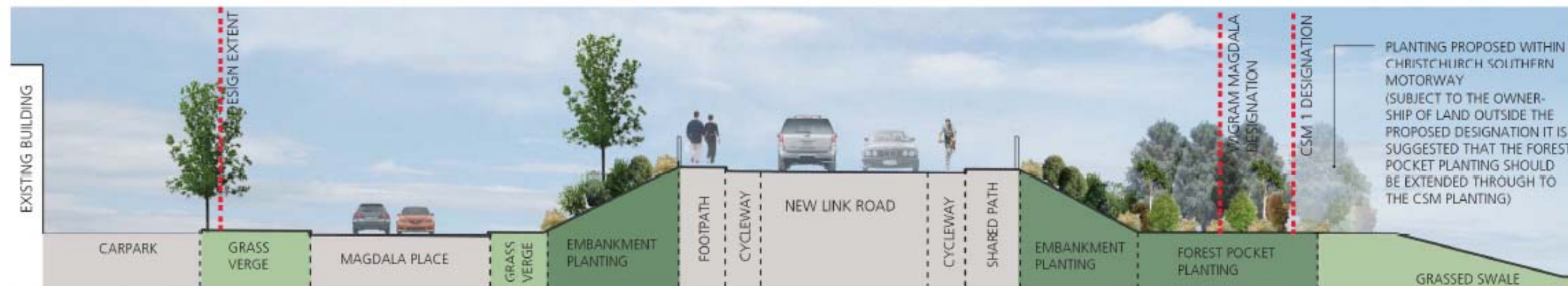
CROSS SECTION B - B' THIS SECTION DEMONSTRATES THE NEW LINK ROAD WITH THE PROPOSED LANDSCAPE TREATMENT. EMBANKMENT PLANTING SEPARATES THE TWO ROADS AND PROVIDES VISUAL SCREENING FOR RESIDENTS AND BUSINESSES ON MAGDALA PLACE
