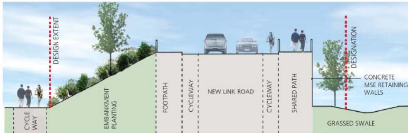
CROSS SECTION A - A' SECTION SHOWS THE RAISED LINK ROAD WITH PROPOSED CYCLEWAY/ FOOTPATH RUNNING ALONG THE BASE OF THE STRUCTURE
