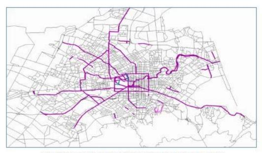
Illustrative Segregated Cycle Path Additions for a 2026 Test model (Note Blenheim Road is a proxy for a Southern Railway cycleway and Main North Rd is a proxy for extension of the Northern Railway Cycleway)
