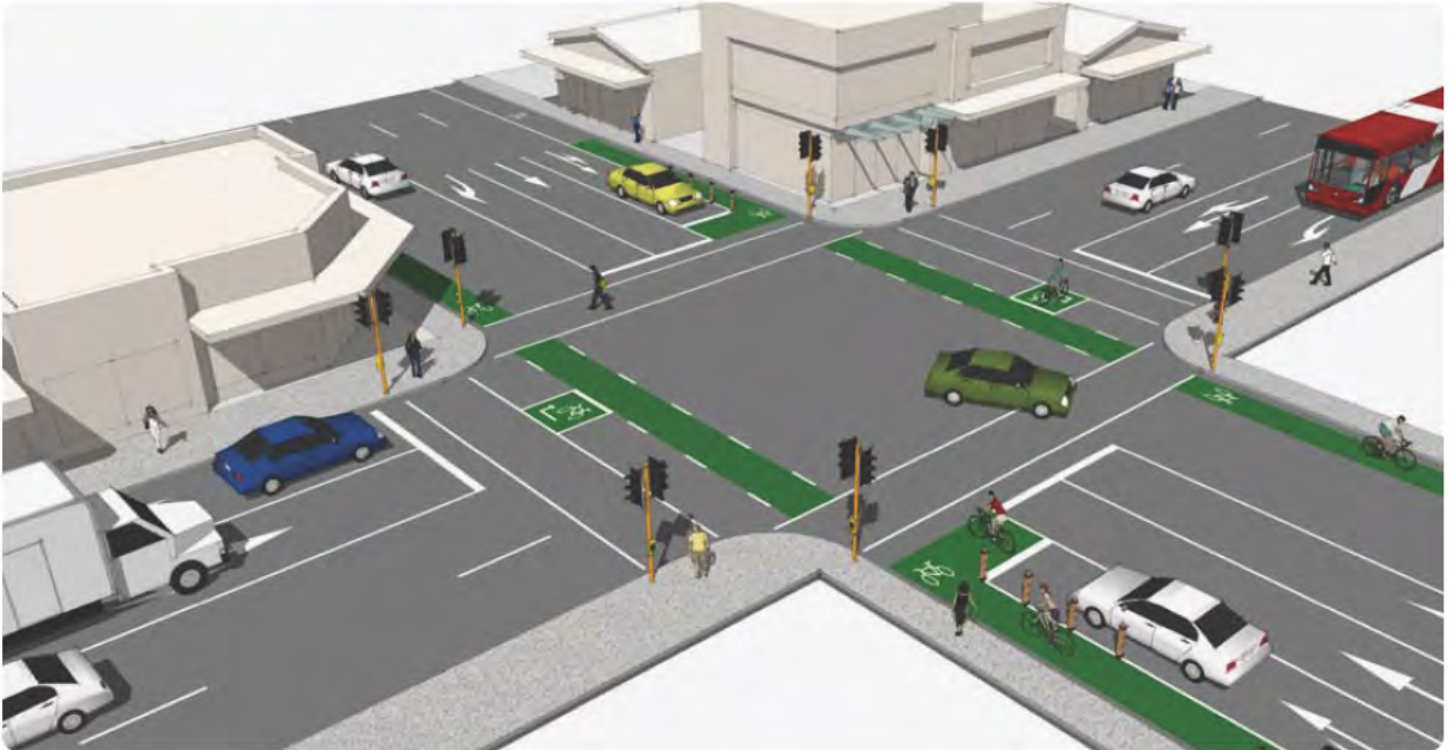
1. Single cycle lane at the intersection.
