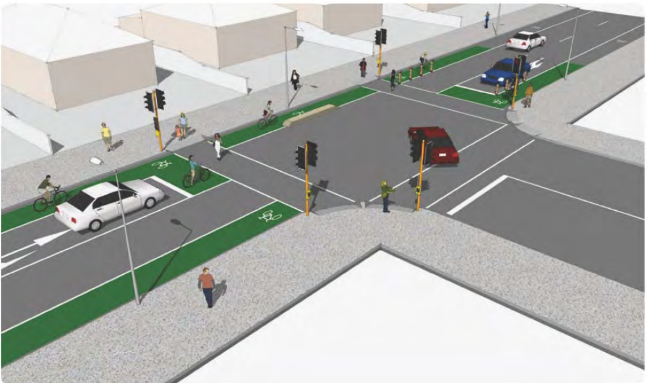
2. Cycle signals allow cycles to continue through the top of the T-intersection.
