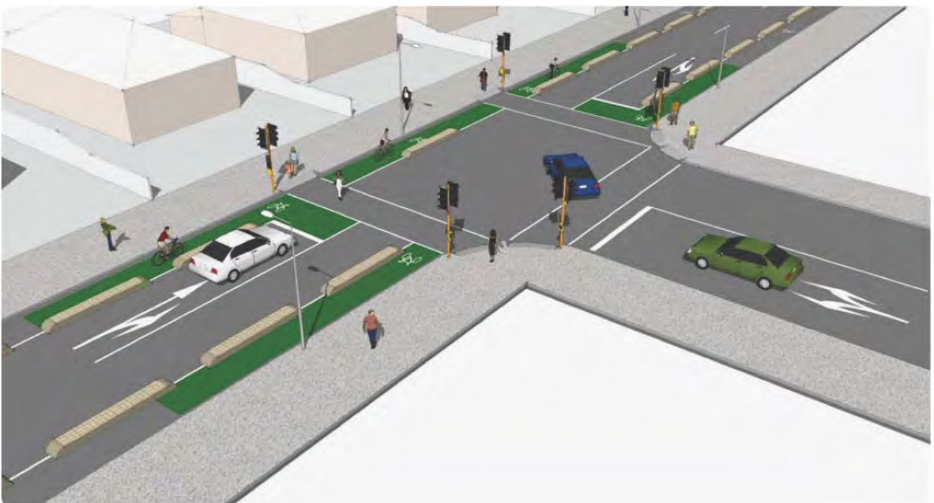
2. T-intersection cycle signals allow cycles to continue through the top of the intersection.
