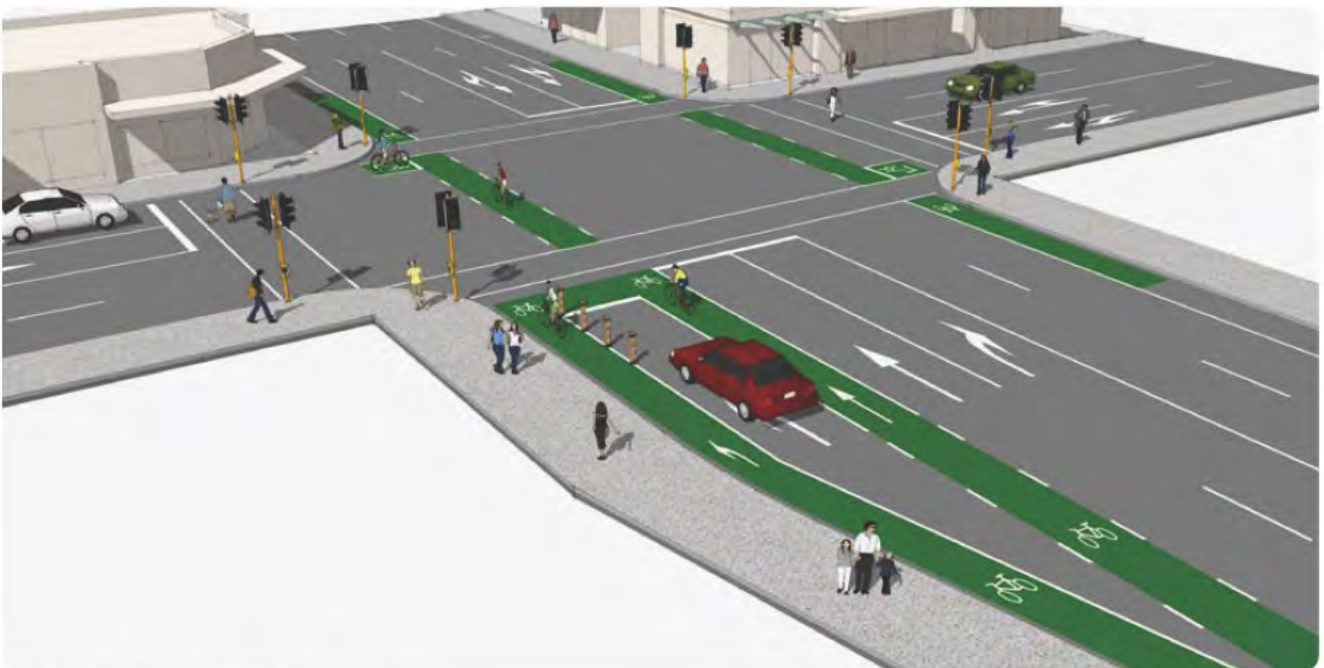
2. Left-turn and straight-through cycle lane at the intersection.
