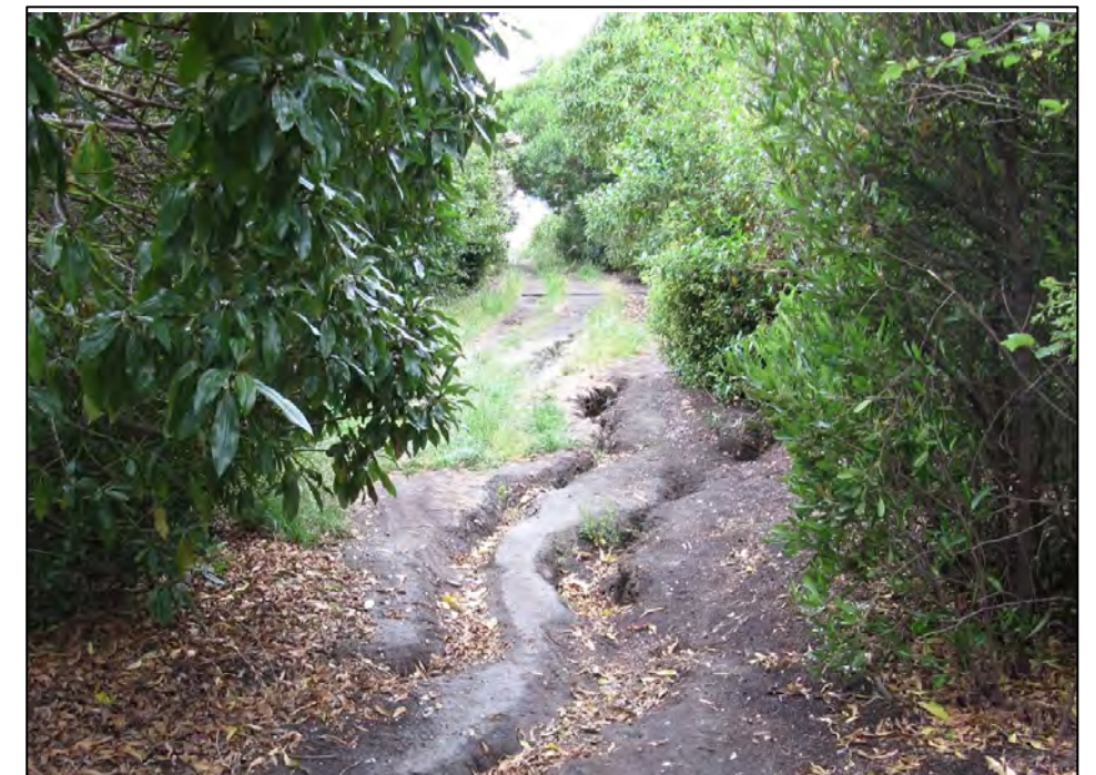
Figure 16: Cracking as a result of lateral spread is clearly seen along the banks of the Heathcote River.
