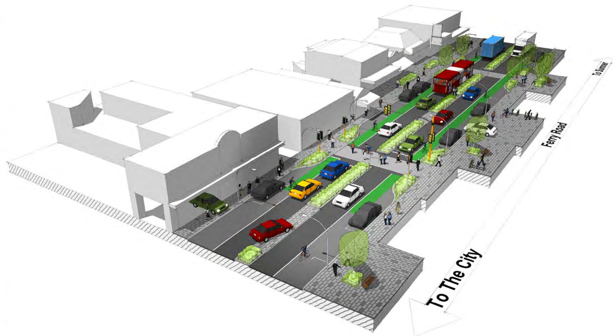
Figure 41: This perspective shows Option 1 for the design of Woolston commercial centre. Improvements to the road corridor include retaining on-street car parking and a separated cycle lane.
