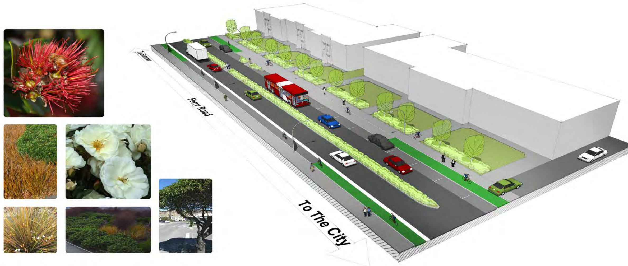
Figure 46: Perspective facing south west, showing road corridor improvements to Ferry Road through Ferrymead, including a separated cycleway and the retention of limited on street parking.
