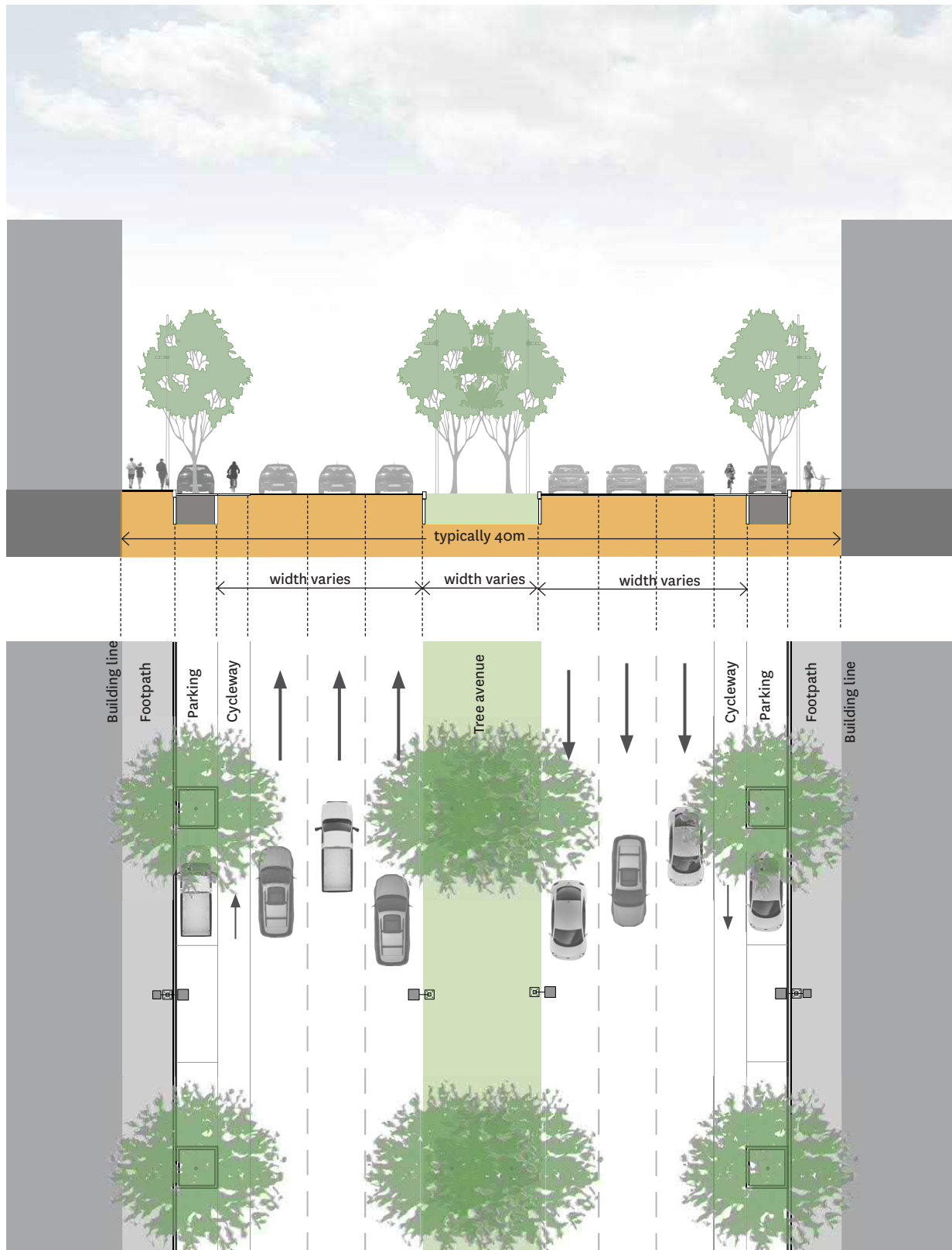
Figure 73 Moorhouse, Bealey and Fitzgerald avenues – typical existing cross-section
